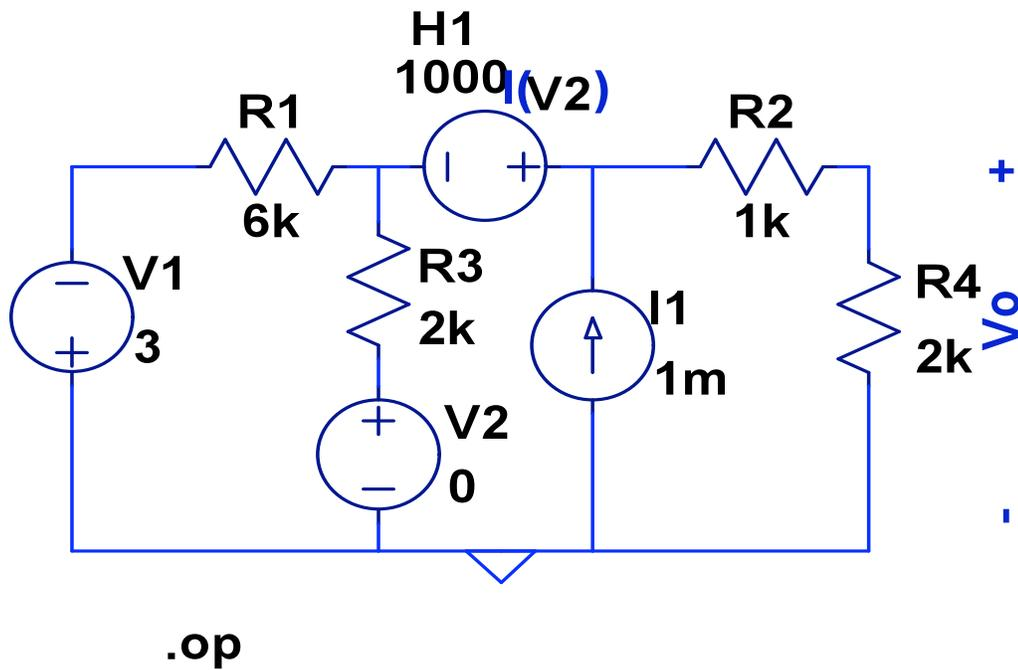
Figure 2. LTSpice Equivalent Circuit
