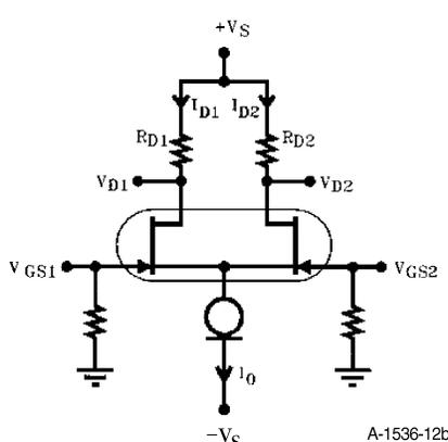
FIGURE 12B: Improved differential amplifier with constant-current source.
