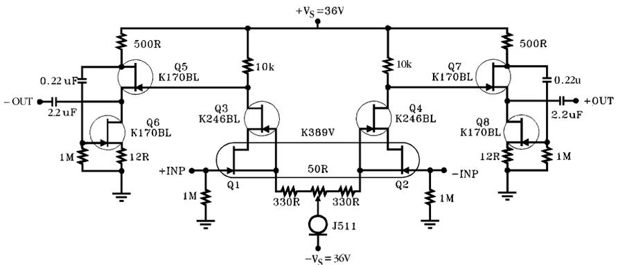
FIGURE 17: The all-JFET balanced SE line amp.
