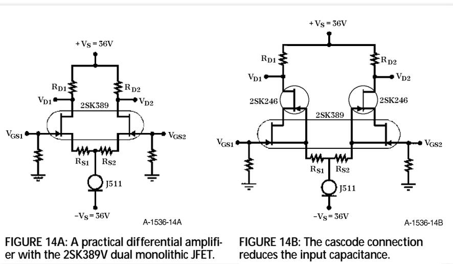
FIGURE 14A: A practical differential amplifier with the 2SK389V dual monolithic JFET.
